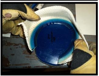
Place the shoe assembly between two plates in the arbor press for a couple minutes as it cools to finish bonding the cuff to the shoe.
