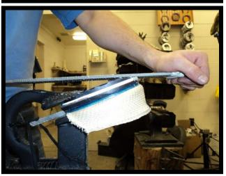
The break-over has now been relieved into the toe of the shoe and all around the ground surface edge.
